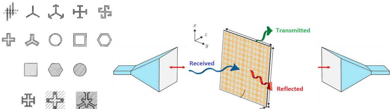
Figure 1. Shapes and principles of FSS
