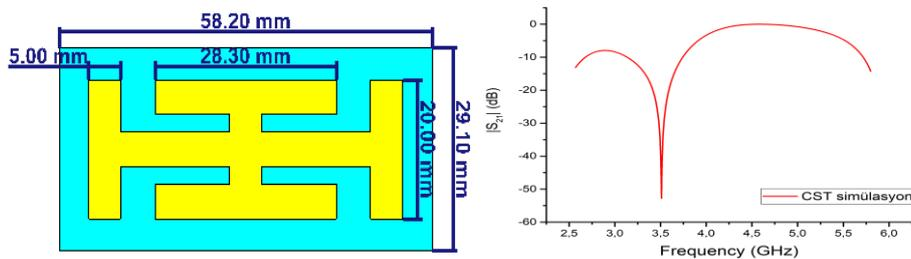
Figure 2. Jarusalem cross unitcell and transmission coefficient
