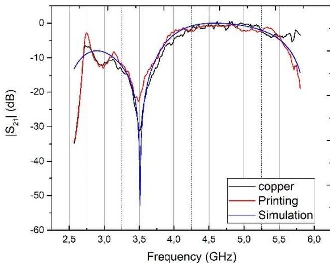
**Figure 7.** S- parametres of screen printing FSS
