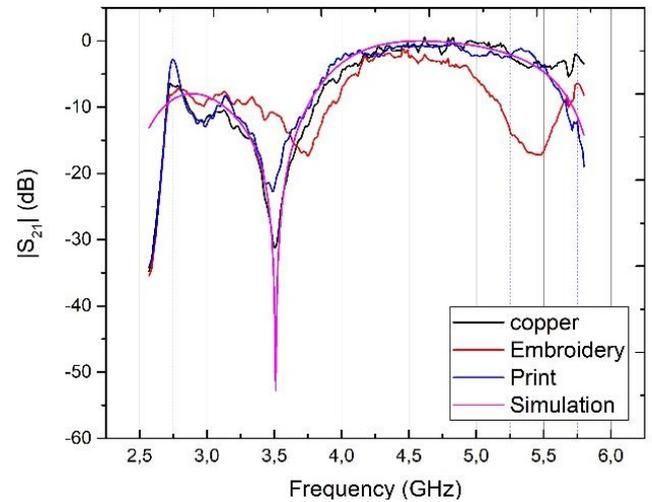
**Figure 8.** Transmission coefficient of textile based FSSs
