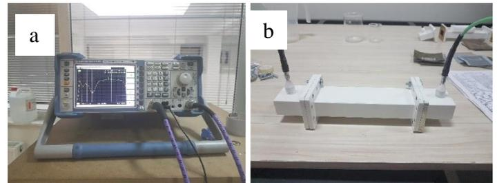
Figure 4. Measurement setup, Network analyzer (a), WR 229 waveguide (b)
