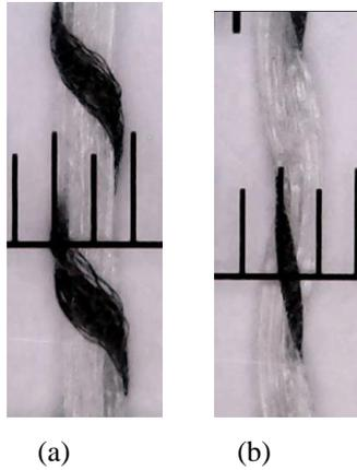
**Figure 2.** Bare HAY without roving (a) without tension (b) under 45% extension.
