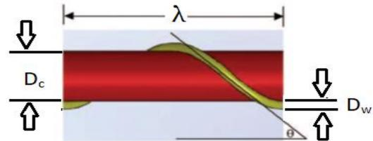
Figure 1. Image of effective diameter measurement of an HAY [2].
