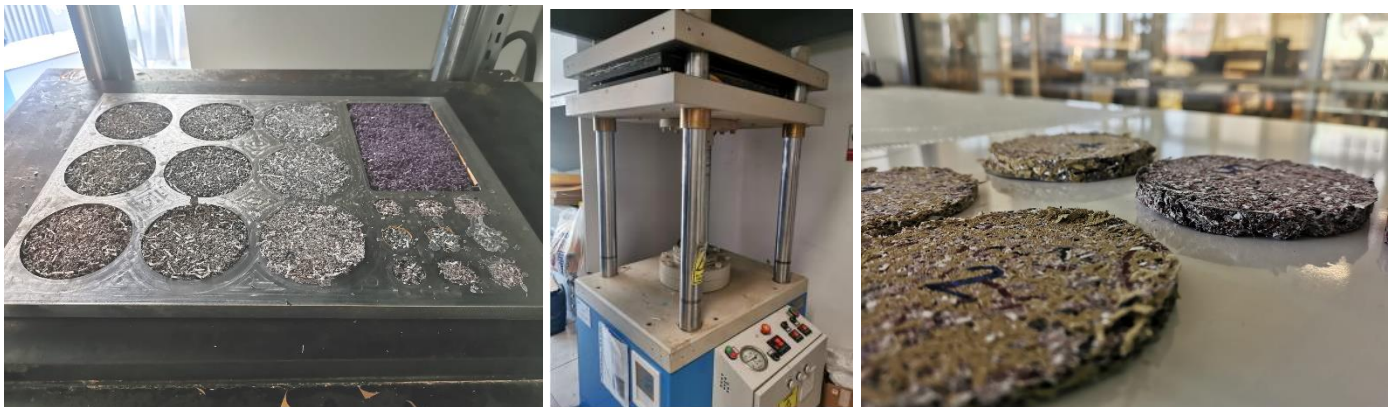
Figure 4. a. the sample placement in a casting mold, b. hot press, c. produced composite samples
