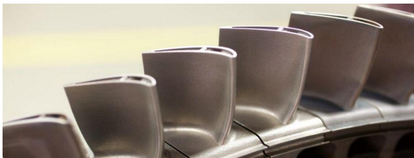
Figure 8. Siemens UK starts additive manufacturing of turbine blades [21]
