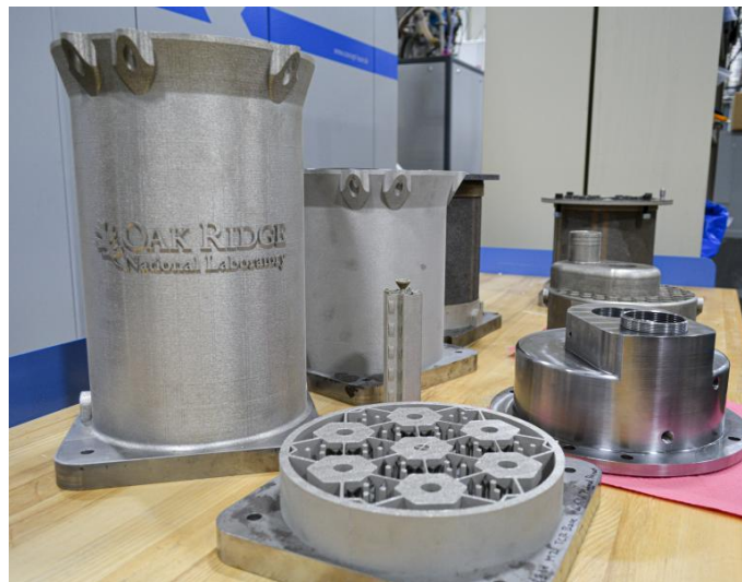
Figure 1. Reactor produced by 3D printing [12]
