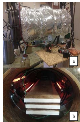
Figure 1. a) Overall view of the kiln during plate heating b) Position of the lumber in the kiln during the IR heating.
