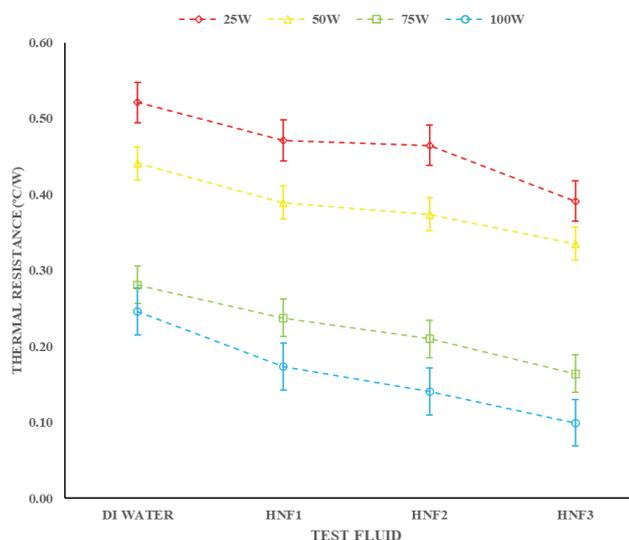
Figure 5. Variation of thermal resistance with heat load.
