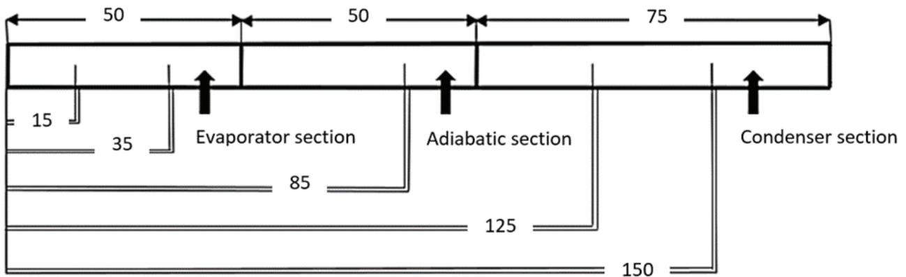
**Figure 2.** Thermocouple placement scheme.
