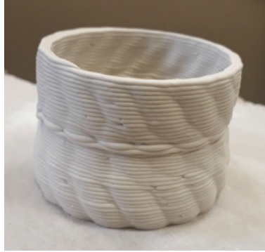
Figure 31. Test using Audrey Blackman Porcelain
