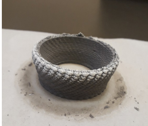
Figure 28. First attempt printing Egyptian paste
