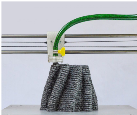
Figure 2. 3D printer that uses recycled paper
