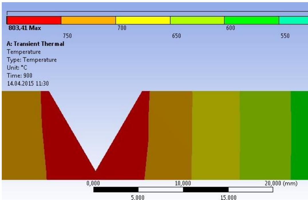
Figure 3. Temperature gradient formed into HAZ
