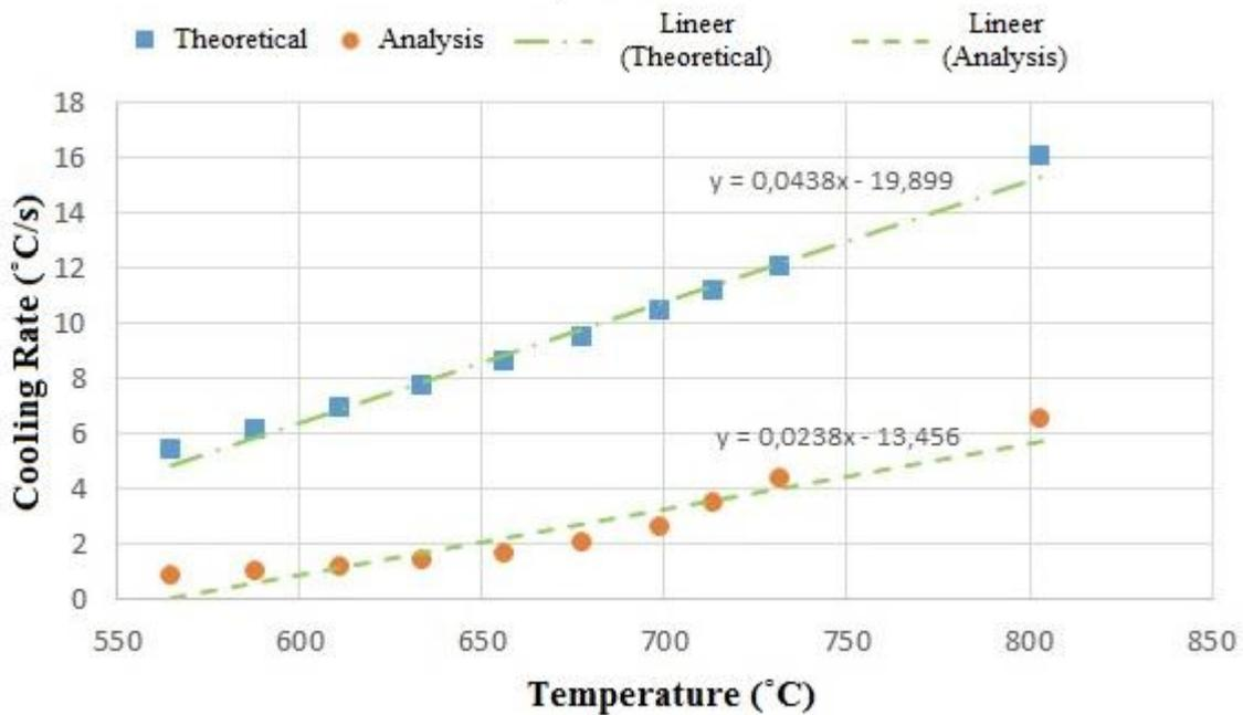
Figure 4. Comparison of theoretical and analysis cooling rates
