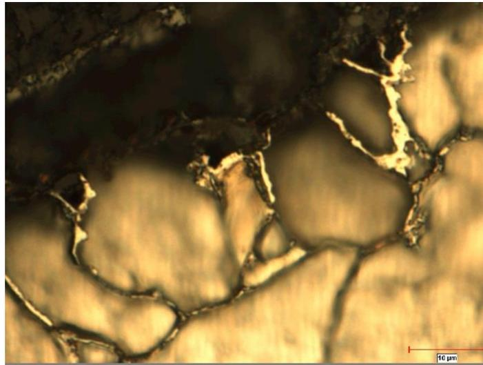
*Figure 3. Industrial sample microstructural view of hot shortness.*
