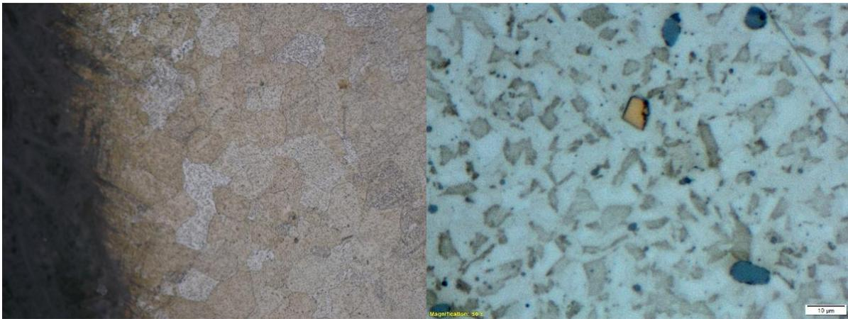
Figure 1. Microstructural view of Scientific 2 (Nital on the left, FeCl<sub>3</sub> on the right).
