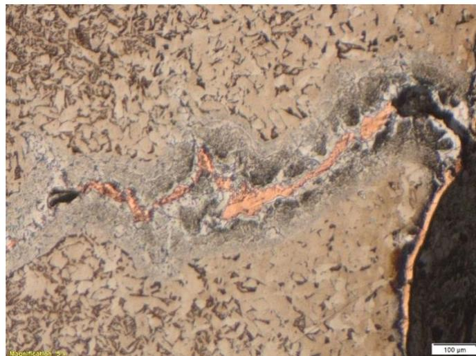
Figure 2. Microstructural view of Scientific 1 etched with FeCl<sub>3</sub> based etchant.
