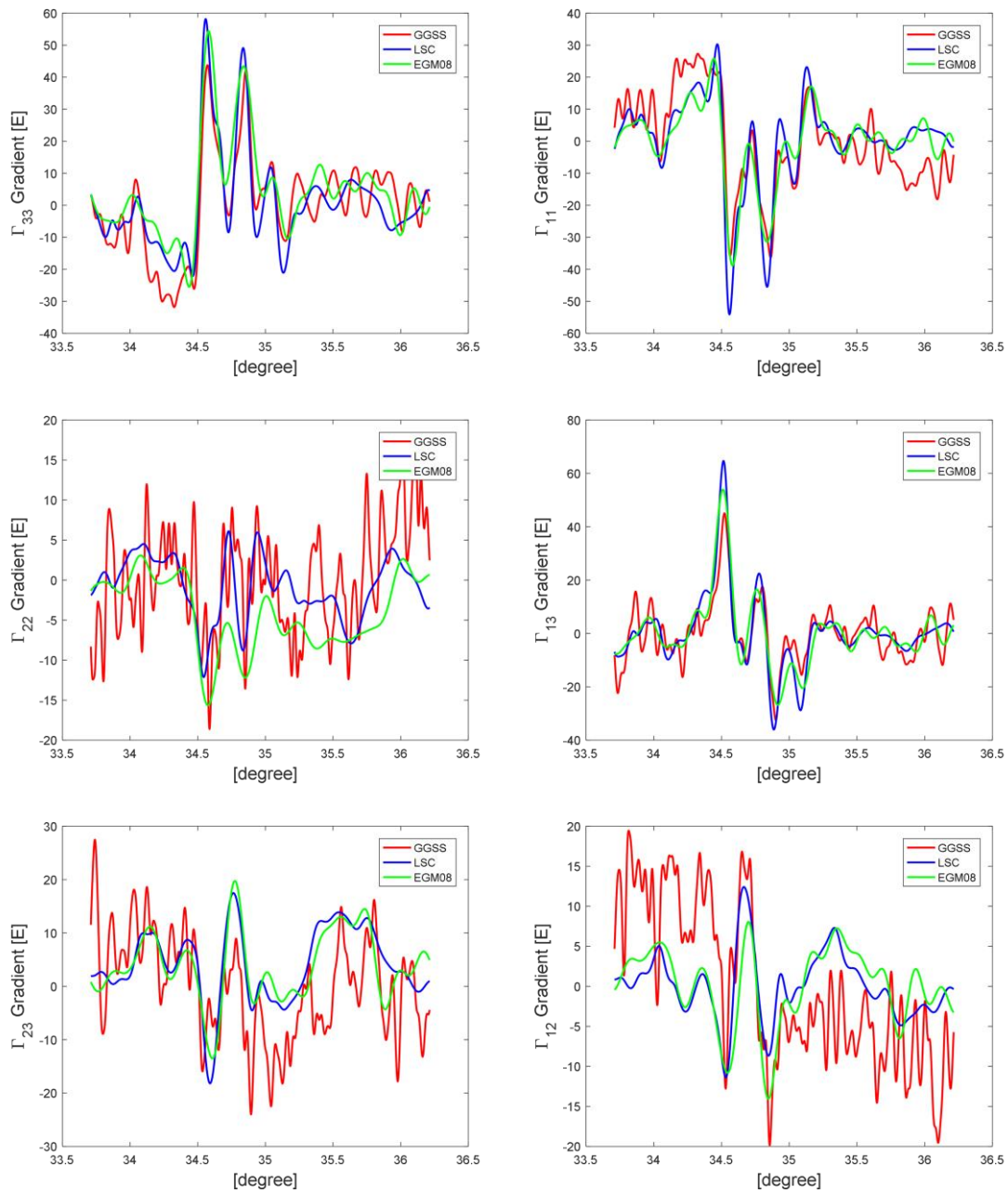
Figure 10. Plots of modeled gravity gradient disturbances, EGM08 gradients and airborne gradiometry data along track T31
