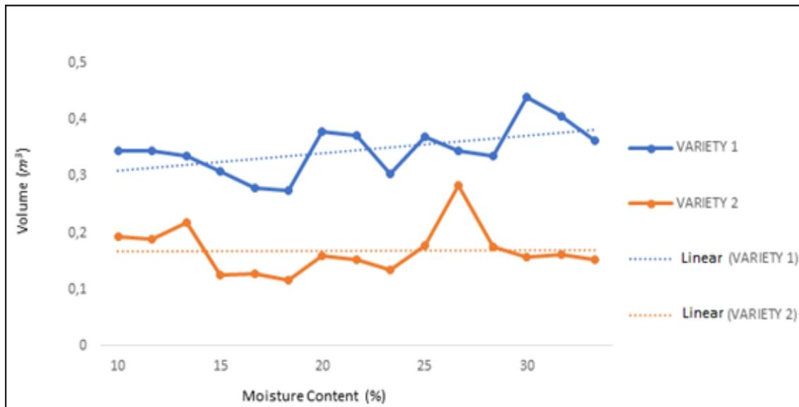
**Figure 1.** Effect of moisture content in % on volume in m<sup>3</sup>.
