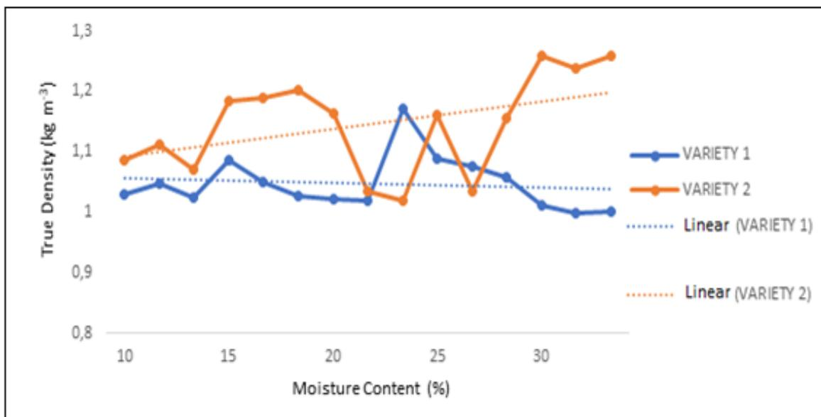
**Figure 3.** Effect of moisture content in % on the true density in  $kg\ m^{-3}$ .
