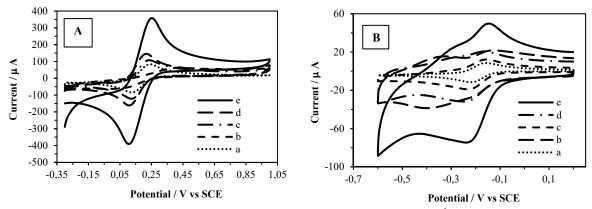
Figure 2. CVs of 2.5 mM  $K_3Fe(CN)_6/K_4Fe(CN)_6$  (A) and 1.0 mM  $Ru(NH_2)_6^{3+}$  (B) obtained with GC (a), GC/ERGO (b), GC/MWCNT (c), GC/A-MWCNT (d) and GC/ERGO/A-MWCNT (e) in 0.1 M KCl. Scan rate: 0.05 V s<sup>-1</sup>.
