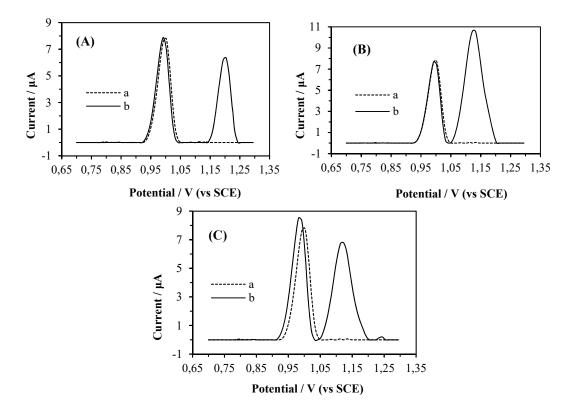
**Figure 4.** DPVs of 2.5 µM LEV in PBS (pH: 2.0) in the absence (a) and presence (b) of 5.0 µM enoxacin (A), ciprofloxacin (B) and norfloxacin (C). Accumulation time: 60 s, Stirring rate 300 rpm.
