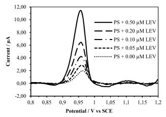
Figure 6. DPVs of GC/ERGO/A-MWCNT in PBS (pH: 2) containing thousand-time diluted pharmaceutical sample in the presence of increasing concentrations of LEV. Accumulation time: 180 s, stirring rate: 300 rpm.
