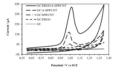
**Figure 1.** CVs of 50.0 μM LEV obtained with different electrodes in 0.1 M PBS (pH: 2.0). Scan rate: 0.05 V s<sup>-1</sup>, accumulation time: 180 s, stirring rate: 300 rpm.
