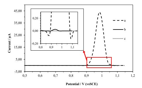
Figure 5. a) DPV of GC/ERGO/A-MWCNT in PBS (pH: 2) containing 5.0 μM LEV. b) DPV of GC/ERGO/A-MWCNT in PBS (pH 2) after waiting the electrode in deionized water for 2 min after performing the measurement a. c) DPV of GC/ERGO/A-MWCNT in PBS (pH 2) after waiting the electrode in PBS (pH 5.0) for 2 min after performing the measurement a. Accumulation time: 180 s, stirring rate: 300 rpm.
