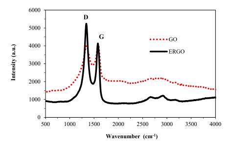
**Figure 3.** Raman spectrums of GO and ERGO obtained with electrochemical reduction via cyclic voltammetry measurements between the potential values of 0.0 V and -1.5 V with a scan rate of 0.05 V s<sup>-1</sup> for 10 scans.
