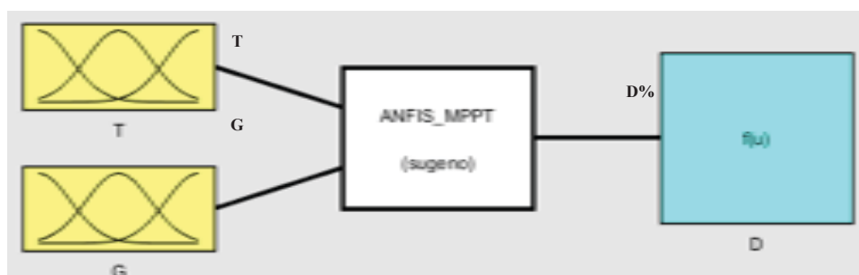
Figure 16. The structure of the generated FLC system after the ANFIS training
