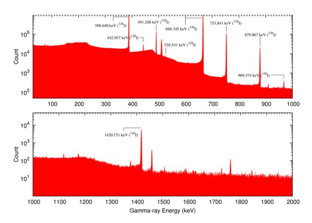
Figure 2. An irradiated <sup>127</sup>I spectrum with bremsstrahlung end-point energy of 18 MeV without background subtraction.
