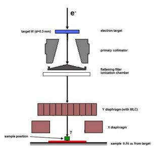
**Figure 1.** Schematic view of the cLINAC setup used for irradiation of <sup>127</sup>I sample.
