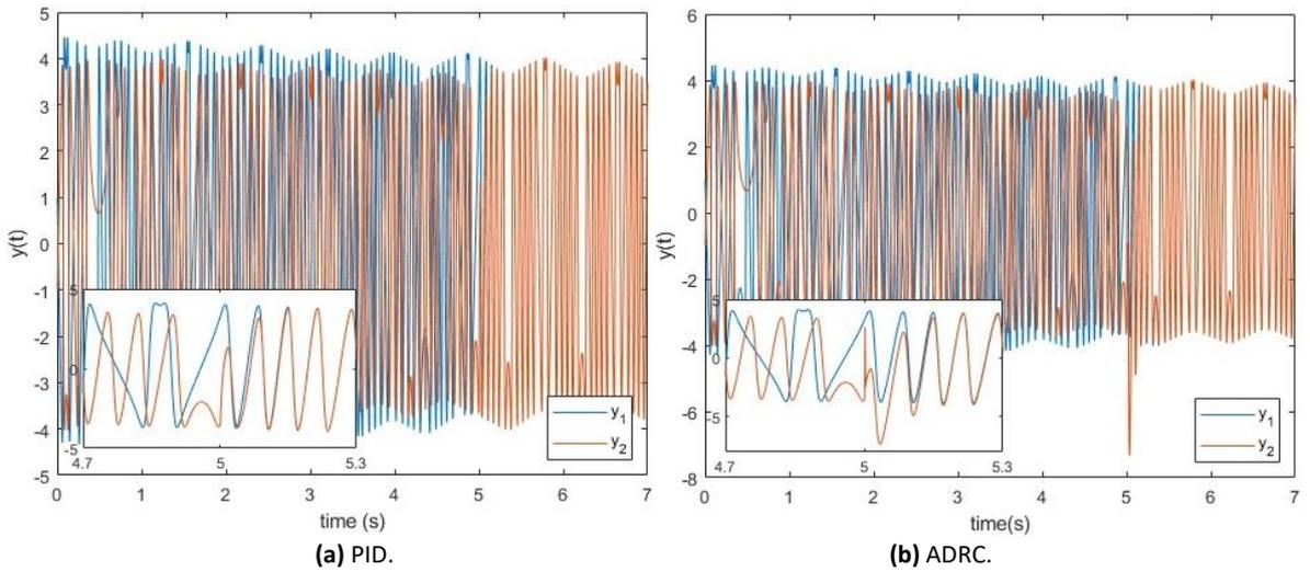
Figure 5. Synchronization of  $y(t)$  function with PID (a) and ADRC (b).
