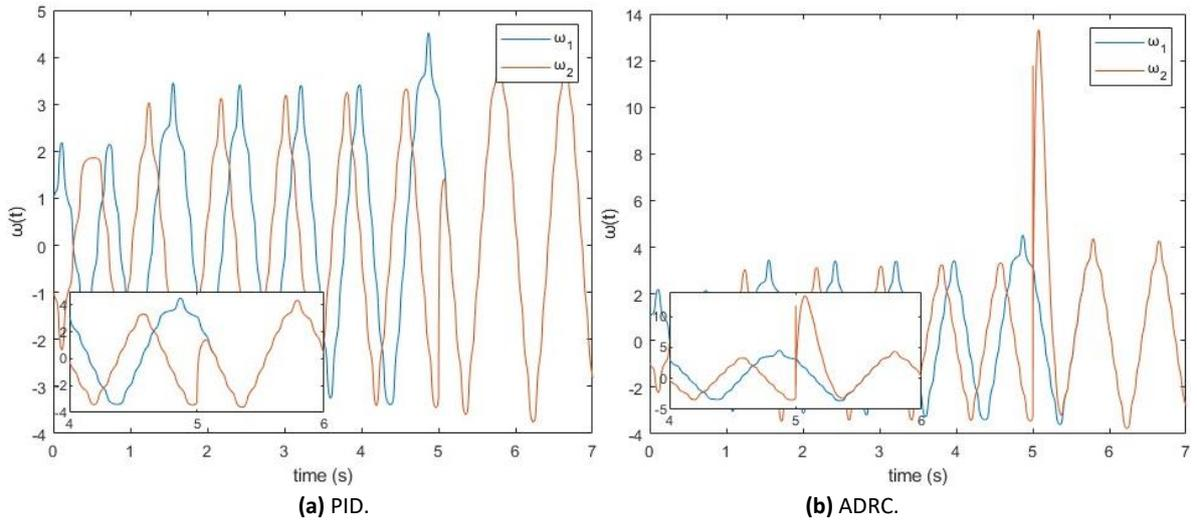
Figure 7. Synchronization of  $\omega(t)$  function with PID (a) and ADRC (b).
