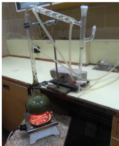
Figure 3. Essential oil isolation by Clevenger apparatus.
