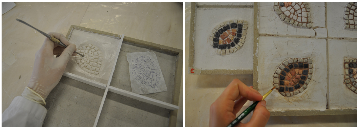
Figure 6 Mortar for engraved tesserae integration - Test with engraved tesserae method (Franzoni 2020).
