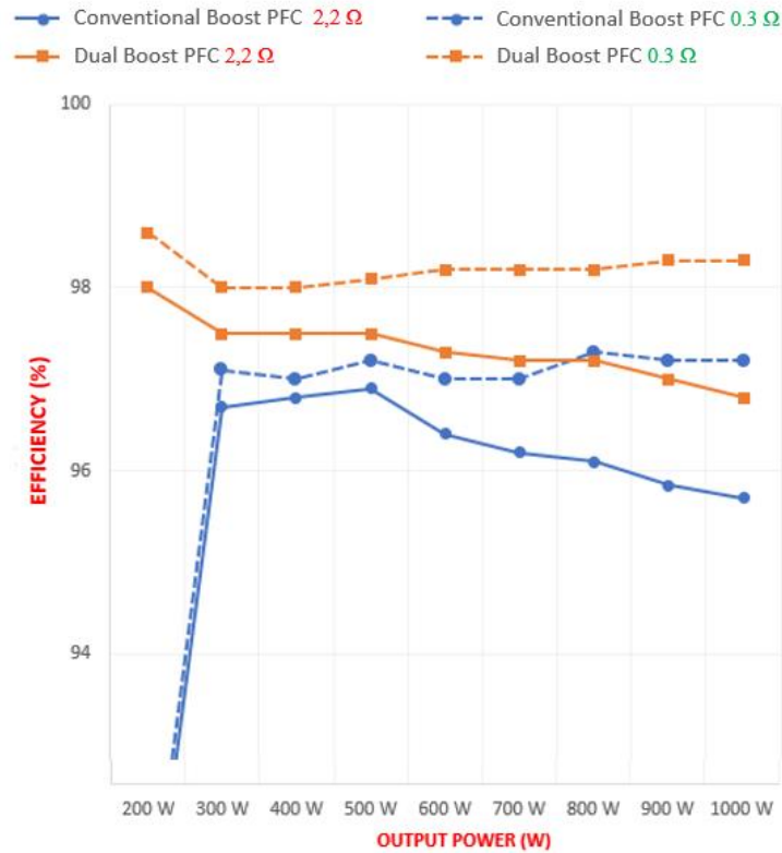
Figure 12. Efficiency graph of Conventional Boost and Dual-Boost Bridgeless PFC converters operated with different switches
