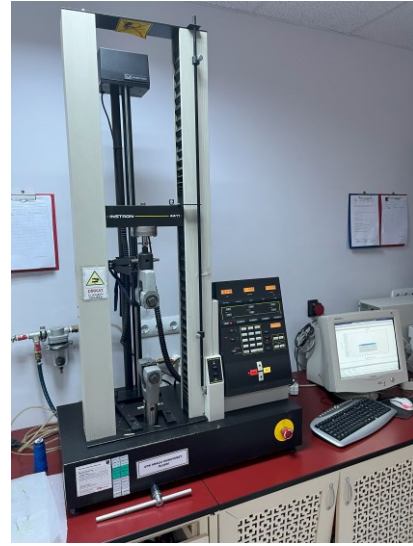
Figure 1. Instron 4411 tensile test machine
