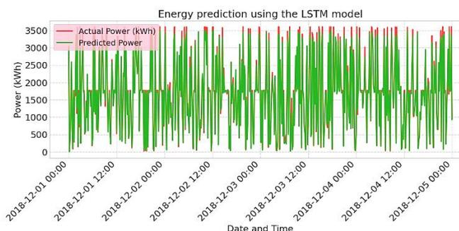
Figure 7. Time slice of predicted and active power
