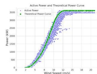
Figure 3. Relationship between actual power and wind speed in the preprocessed data set
