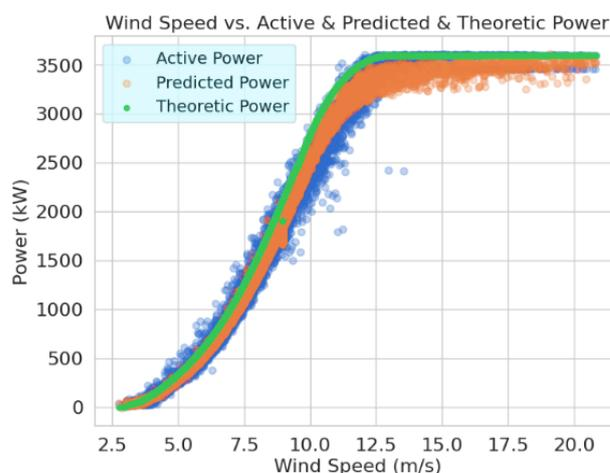
Figure 6. Graph of theoretical, active, predicted power and wind speed
