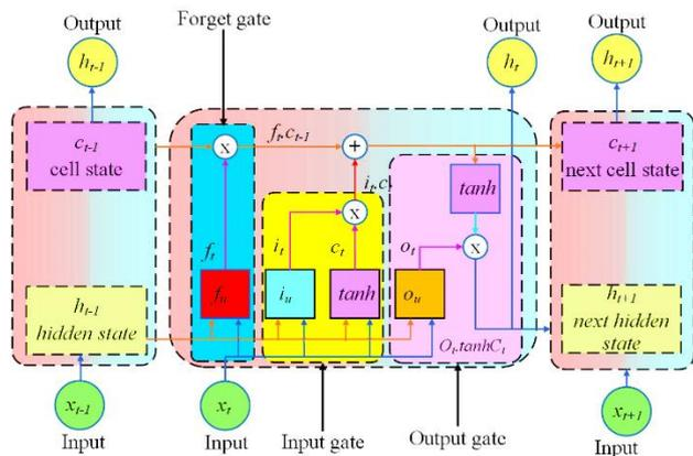
Figure 4. Basic structure of the LSTM model [57]
