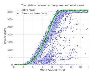
Figure 2. Relationship between actual power and wind speed in the raw data set
