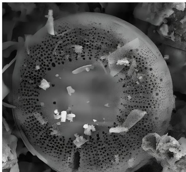
Figure 1. Electron microscope image of the general structure of the diatomaceous earth used in the study.
