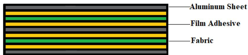
**Figure 4.** Al sheets, hybrid fabrics and adhesives sequences
