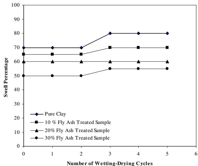
Fig. 8. Variation of Free Swell with Cyclic Wetting-Drying
