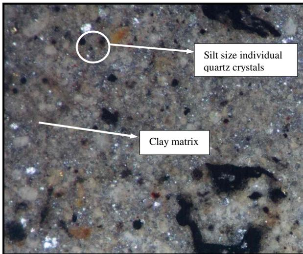
Fig. 1. Micrograph Photo of Pure Clay (Xpol., Obj.x4, Oc.x4).
