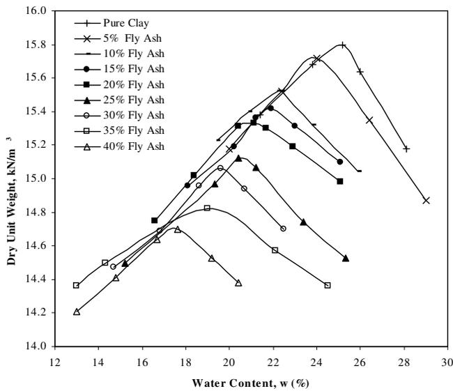
Fig. 5. Standard Proctor Compaction Curves of the Mixtures
