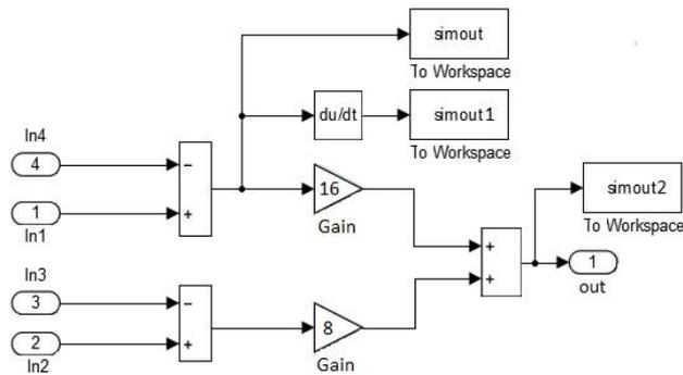
**Figure 8.** The inner structure of PD controller.
