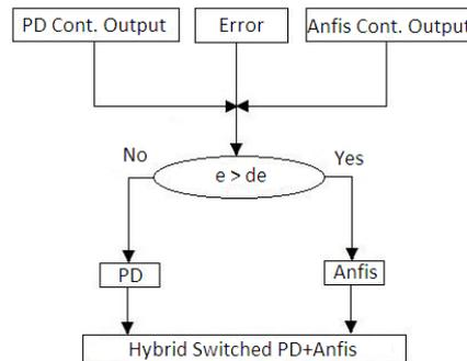
Figure 5. The control block diagram of hybrid switched PD+Anfis controller.
