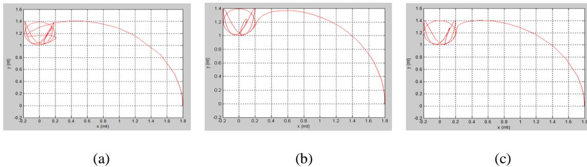
**Figure 16.** Robot's end point in x-y coordinates for the hybrid trajectory: (a) PD controller, (b) Anfis controller, (c) Hybrid PD+Anfis controller.
