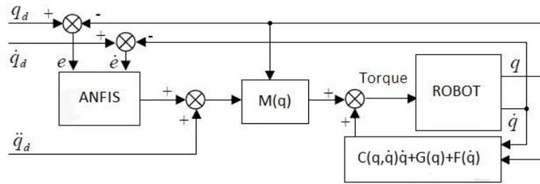
Figure 4. Anfis control block diagram of the robot arm.
