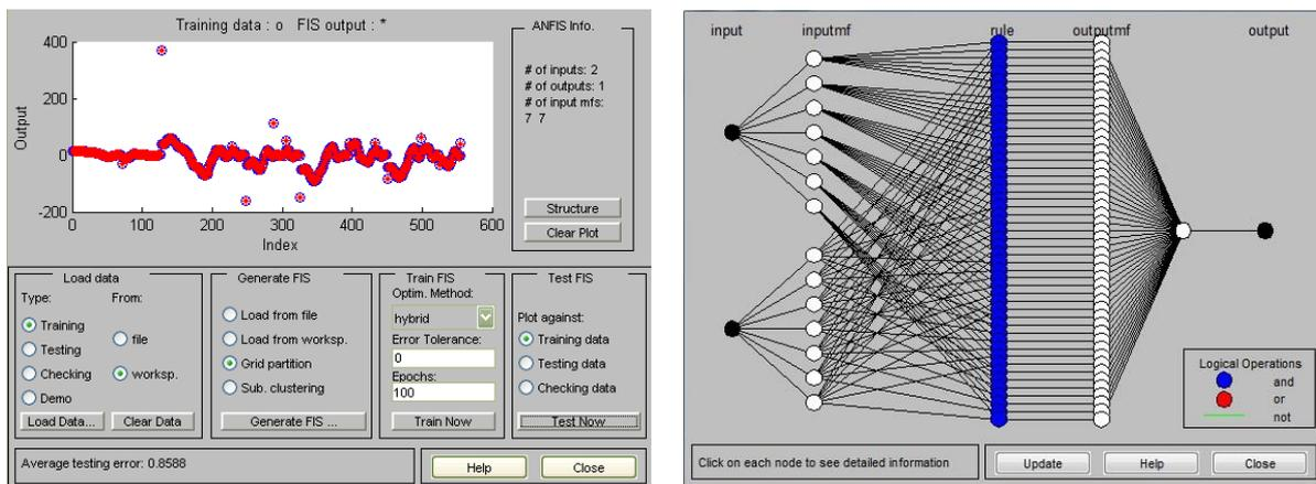
**Figure 9.** (a) Training of data received from PD controller with Anfis, (b) 5 layered general structure of Anfis.
