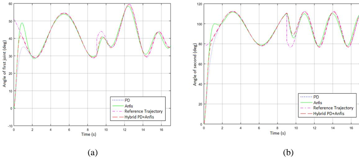
**Figure 15.** (a) The angle of the first joint in a hybrid trajectory, (b) The angle of the second joint in a hybrid trajectory.
