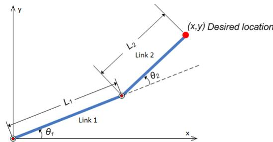
Figure 1. The model of two DOF robot arm.
