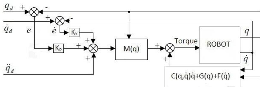
Figure 2. PD control block diagram of the robot arm
