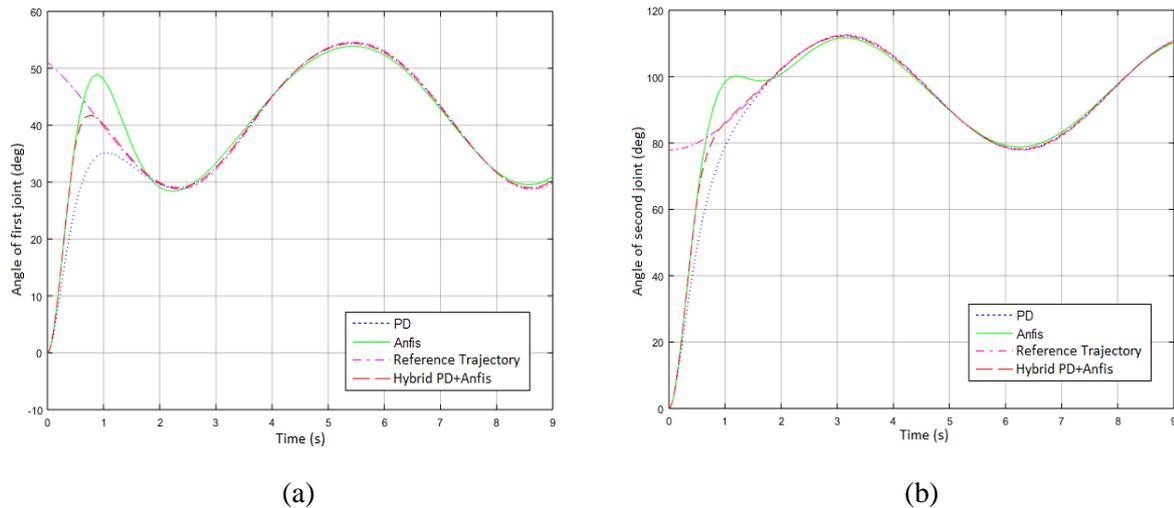
**Figure 13.** (a) Angle value of the first joint in a circular trajectory, (b) Angle value of the first joint in a circular trajectory.
