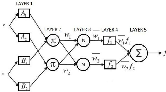
**Figure 3.** The architecture model of Anfis.
