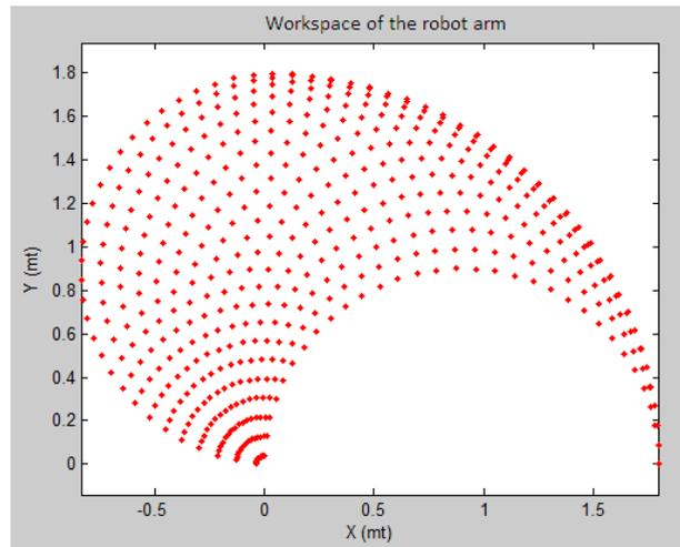
Figure 6. The workspace of two DOF robot arm.
