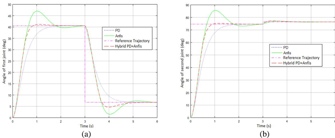
**Figure 11.** (a) The angle value of the first joint for a switched trajectory, (b) The angle value of the second joint for a switched trajectory.
