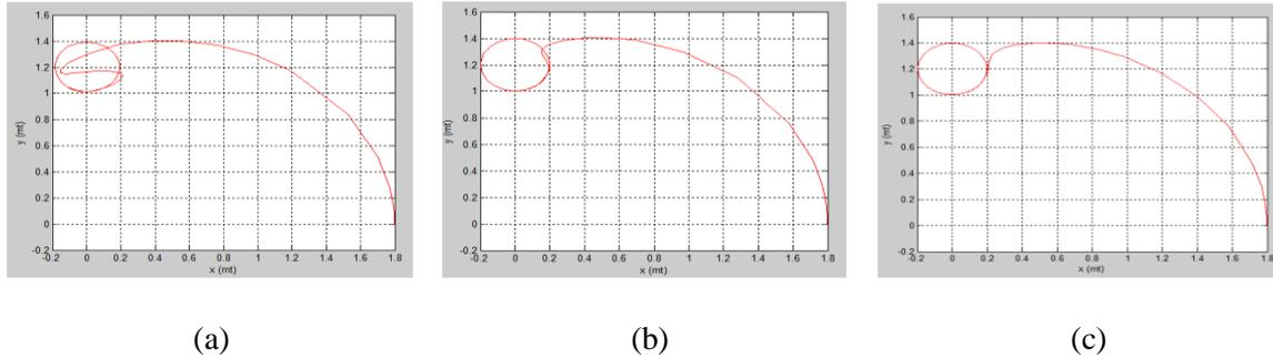
**Figure 14.** Robot's end point in x-y coordinates for the circular trajectory: (a) PD controller, (b) Anfis controller, (c) Hybrid PD+Anfis controller.
