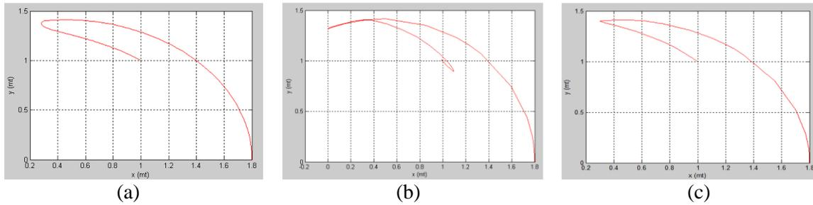
**Figure 12.** Robot's end point in x-y coordinates for the switched trajectory: (a) PD controller, (b) Anfis controller, (c) Hybrid Switched PD+Anfis controller.
