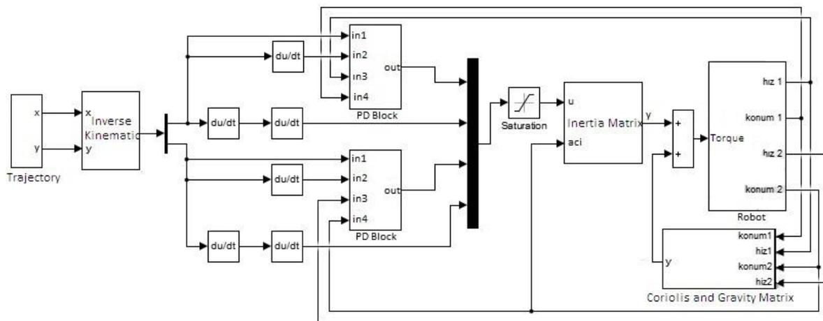
Figure7. The PD control block diagram of two DOF robot arm.
