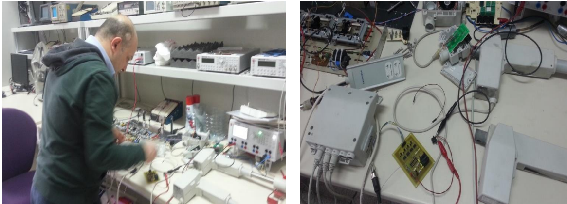
Figure 9. The disassembling process of the motors and the control unit of a sickbed.
