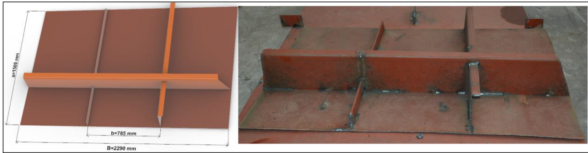
Figure 12. Fabricated stiffened plate and FEM model.
