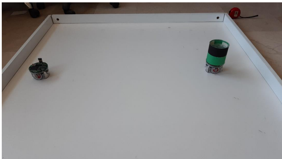
Figure 2. Two e-puck robots on the experimental setup. The one on the left is programmed as a tracker and the one on the right as a demonstrator.
