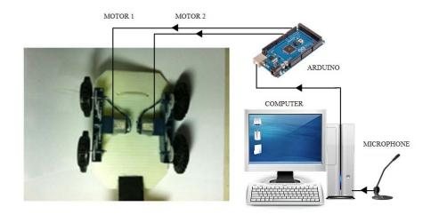
Figure 1. Mechanic drive system of the SCR
