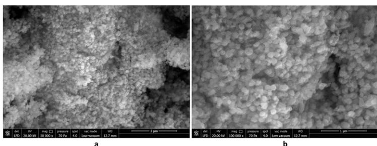
**Figure 3.** SEM microscopy of O-ZnO nanoparticles at different magnifications: a) x 50 k, b) x 100 k
