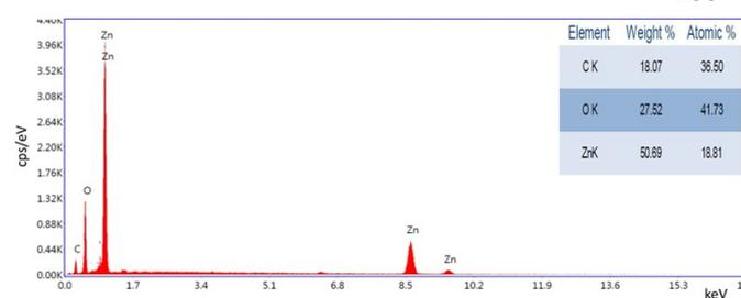
**Figure 4.** EDX spectrum of O-ZnO NPs.
