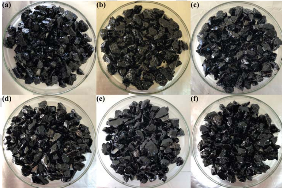
Figure 4 - Images of the samples after the Nicholson stripping test: (a) SBS, (b) SBS+1W, (c) SBS+3W, (d) SBS+5W, (e) SBS+7W, and (f) SBS+9W
