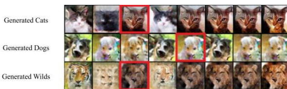
Figure 7. Mode collapse observed with synthetic images generated the latent space dimension z=1 of DCGAN trained with three separate datasets.
