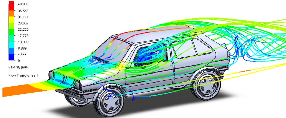
*Figure 6. Velocity distribution of the front side glass opened*
