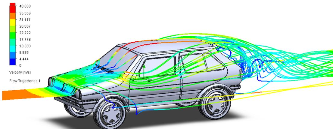
**Figure 2.** Velocity distribution of all glass closed
