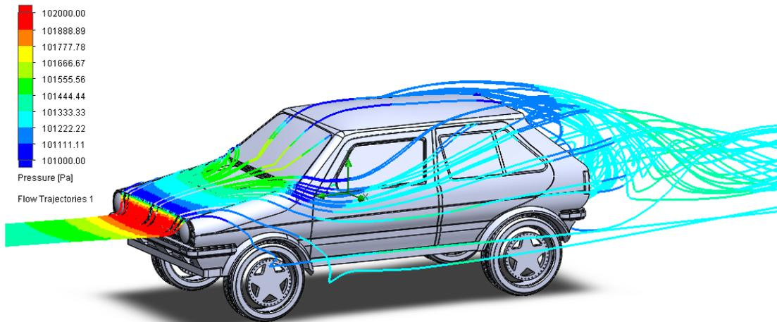
Figure 3. Pressure distribution of on all glass closed
