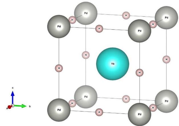
**Figure 1.** The crystal structure representative of YbPdH<sub>3</sub>.
