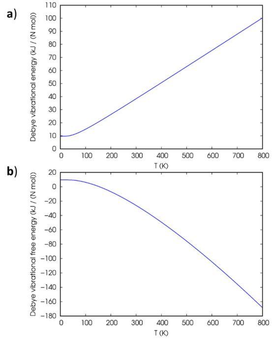
**Figure 5.** Debye vibrational energy (a) and free energy (b) of YbPdH<sub>3</sub>.
