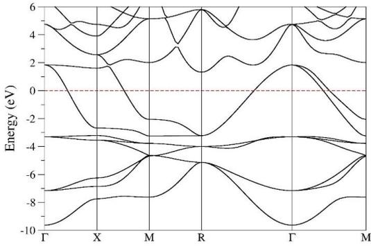
**Figure 3.** Electronic band structure of YbPdH<sub>3</sub>.
