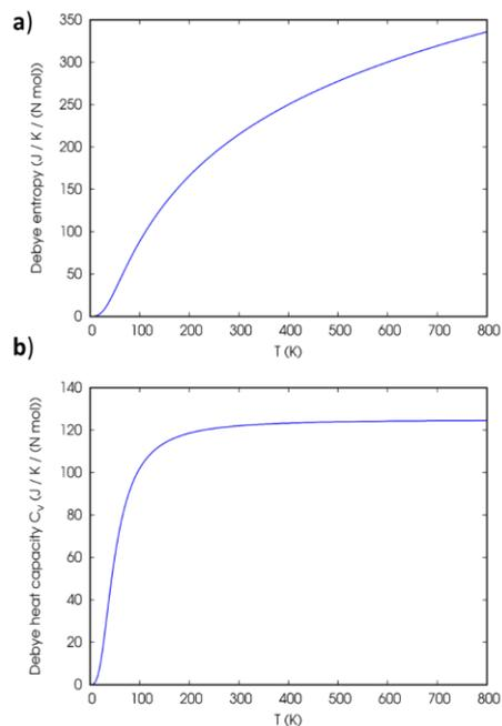
**Figure 6.** Debye entropy (a) and heat capacity (b) of YbPdH<sub>3</sub>.
