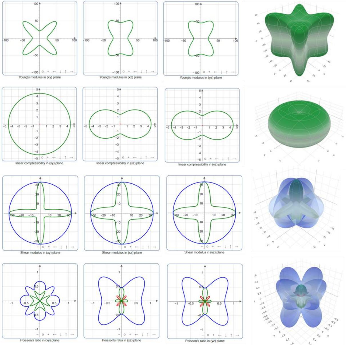
**Figure 2:** The 2D and 3D directional change of Young Modulus, linear compressibility, Shear modulus and Poisson's ratio of YbPdH<sub>3</sub>.
