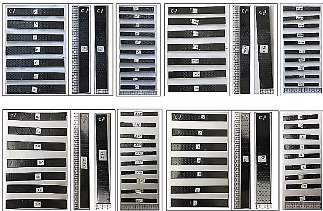
Fig. 3. CFRP composite tensile and three-point bending test specimens with different orientation angles of C_1^8 , C_2^8 , C_3^8 and C_4^8
