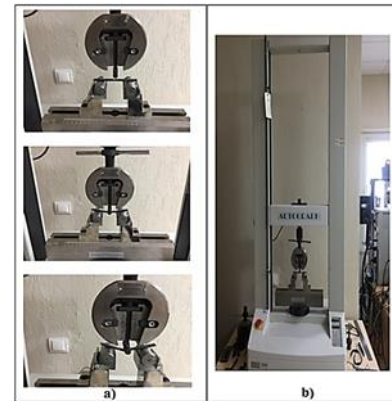
Fig. 4. a) Three-point bending test of the prepared test samples b) AUTOGRAPH device.
