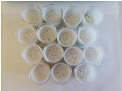
**Figure 1.** hBN coated PA 66/GF30 granules.
