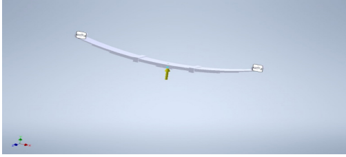
Figure 3. Leaf spring model with load for computer-aided stress analysis
