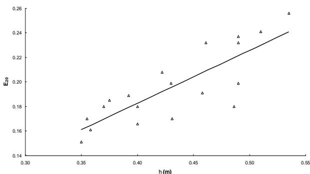
**Figure 2.** Aeration efficiency E<sub>20</sub> versus fall height h.
