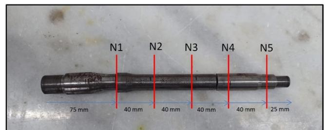
Figure 3. Cross-sectional sampling areas along the barrel length and sample codes
