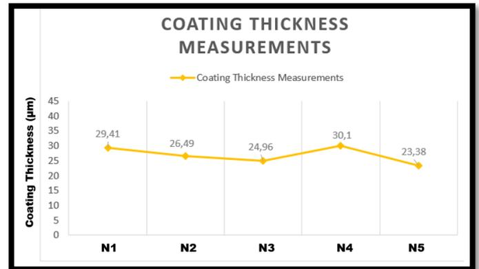
Figure 7. Coating thickness variation along the barrel length
