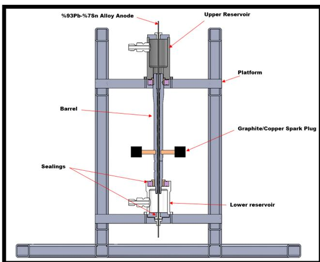
Figure 2. Electroplating cell
