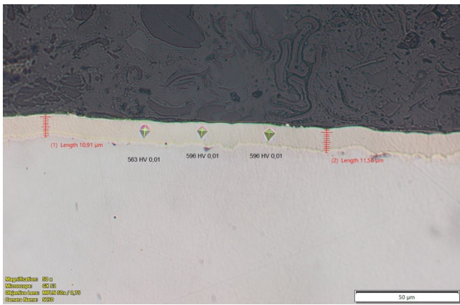
Figure 3. Coating microhardness and coating thickness measurements of the sample EN-1
