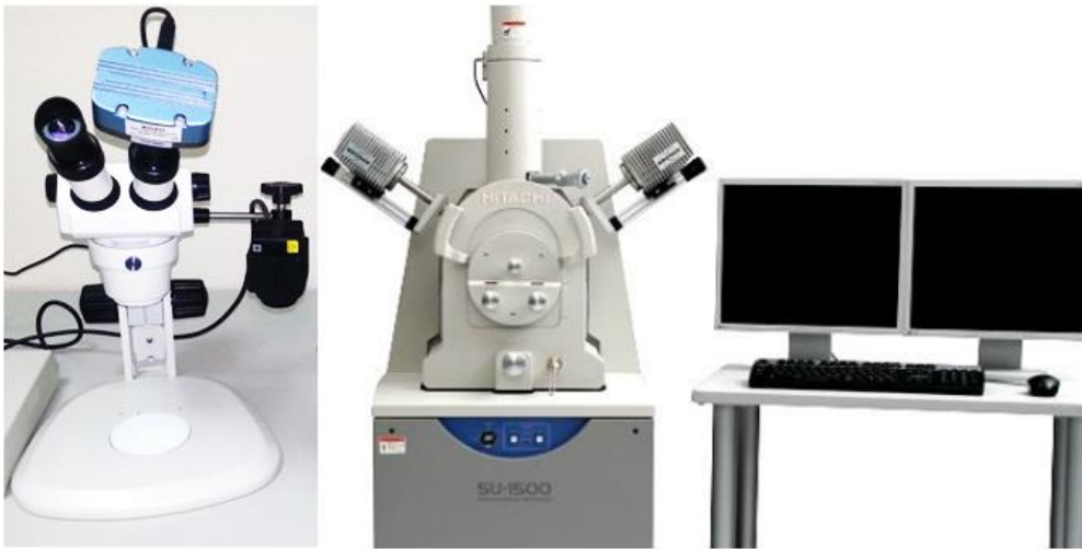
Figure 4. Optical microscope and SEM device used for damage analysis
