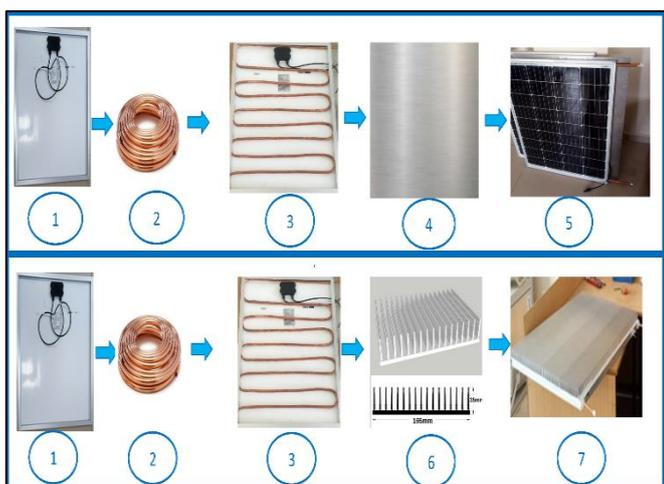
**Figure 3.** Preparation Process of Panels with Cooling. 1- PV panel 2- Copper tube 3- Copper tube mounting behind the panel 4- Metal plate 5- AC panel 6- Aluminum led heatsink 7- HC panel
