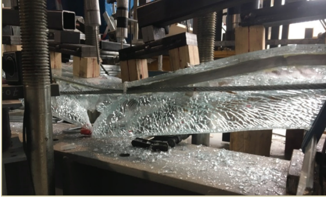
Fig. 21 - Post-tensioned tempered glass T-beam after fracture.
