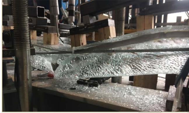
Fig. 21 - Post-tensioned tempered glass T-beam after fracture.
