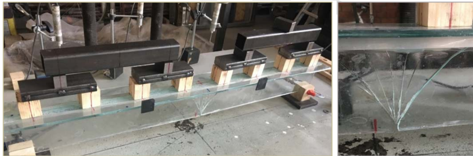
Fig. 16 - Float glass T-beam exposed to its cracking load
