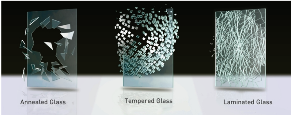
Fig. 1 - Typical fracture shapes of glass types [1]
