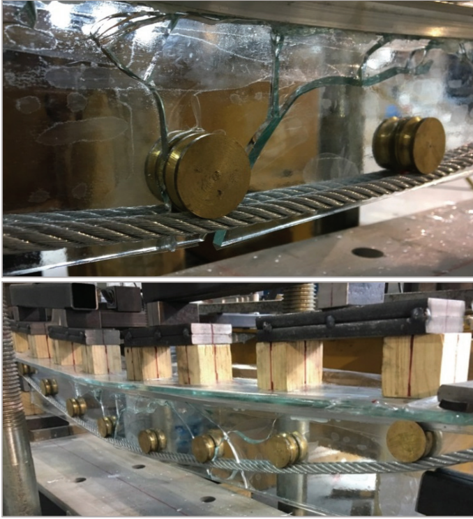
Fig. 19 - Float glass T-beam with post-tensioning after the fracture.
