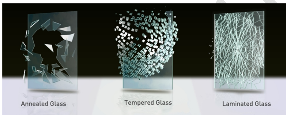
Fig. 1 - Typical fracture shapes of glass types [1]
