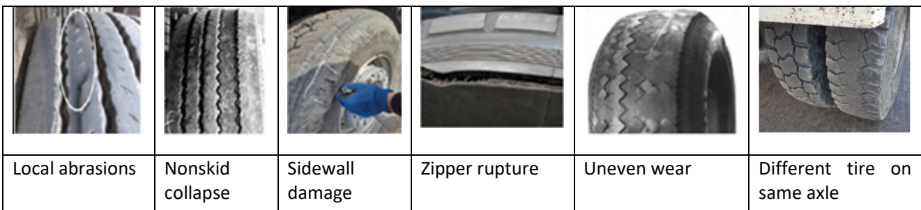
Figure 5. Different types of tire damage
