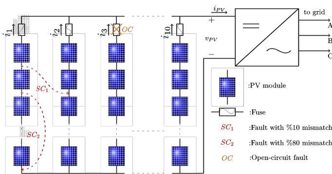
Fig.3. Simulated PV array with potential SC and OC faults [2].
