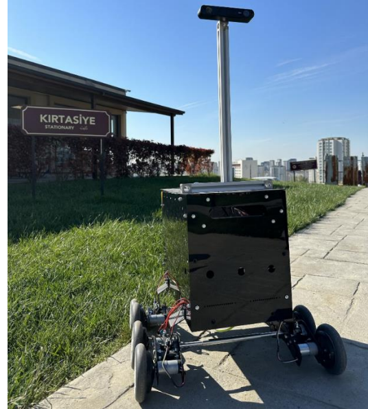
Figure 4. Mobile robot with vision system.
