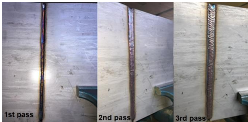
Figure 2. Application of the welding process to plates.
