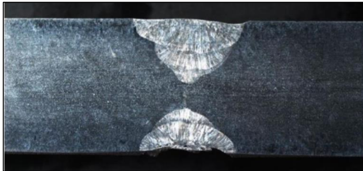
Figure 7. Macrostructure of the plate welded with 150 A.
