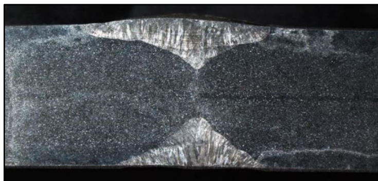
Figure 8. Macrostructure of the plate welded with 175 A.
