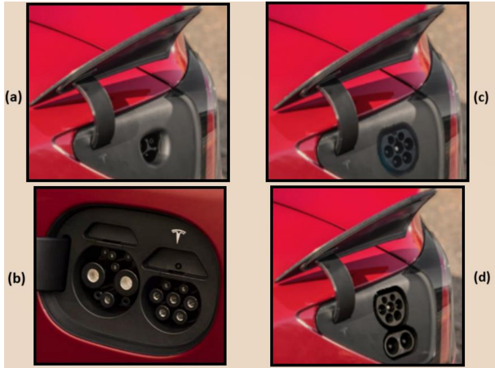
Figure 13. Tesla inlet structure by regions: (a) U.S.; (b) China; (c) Europe and (d) Europe (Rachid et al., 2022)
