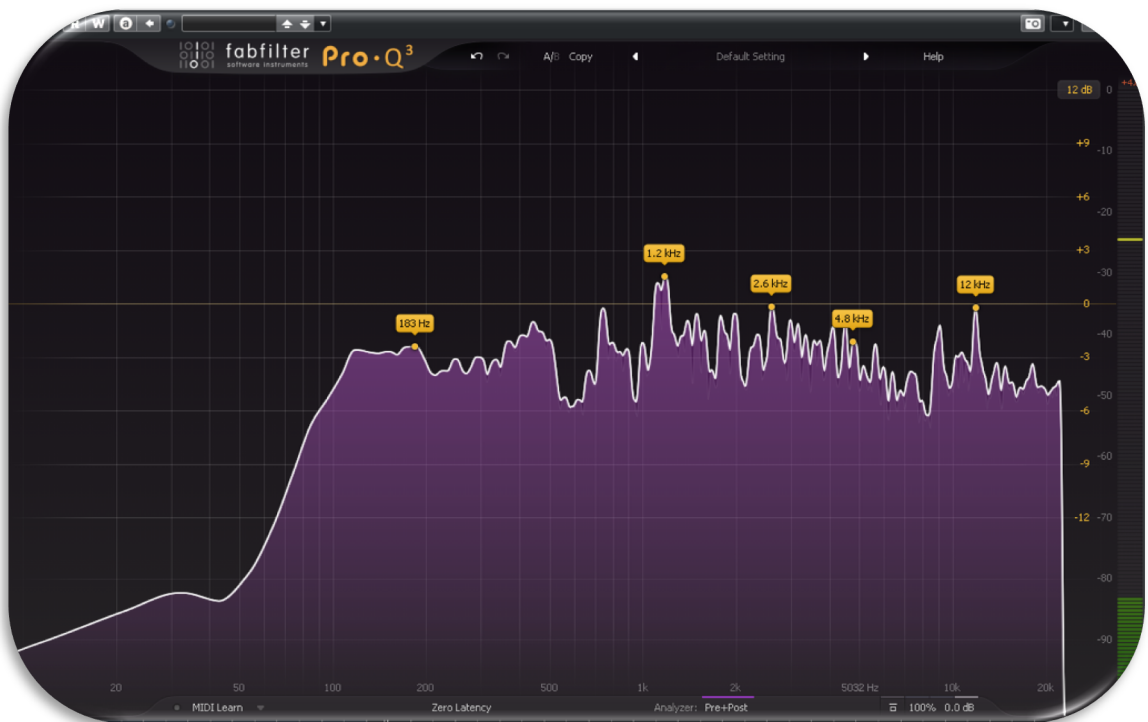
Picture 15. Spectrum analysis of the guitar with the Fabfilter Pro-Q3 plugin (Software)
