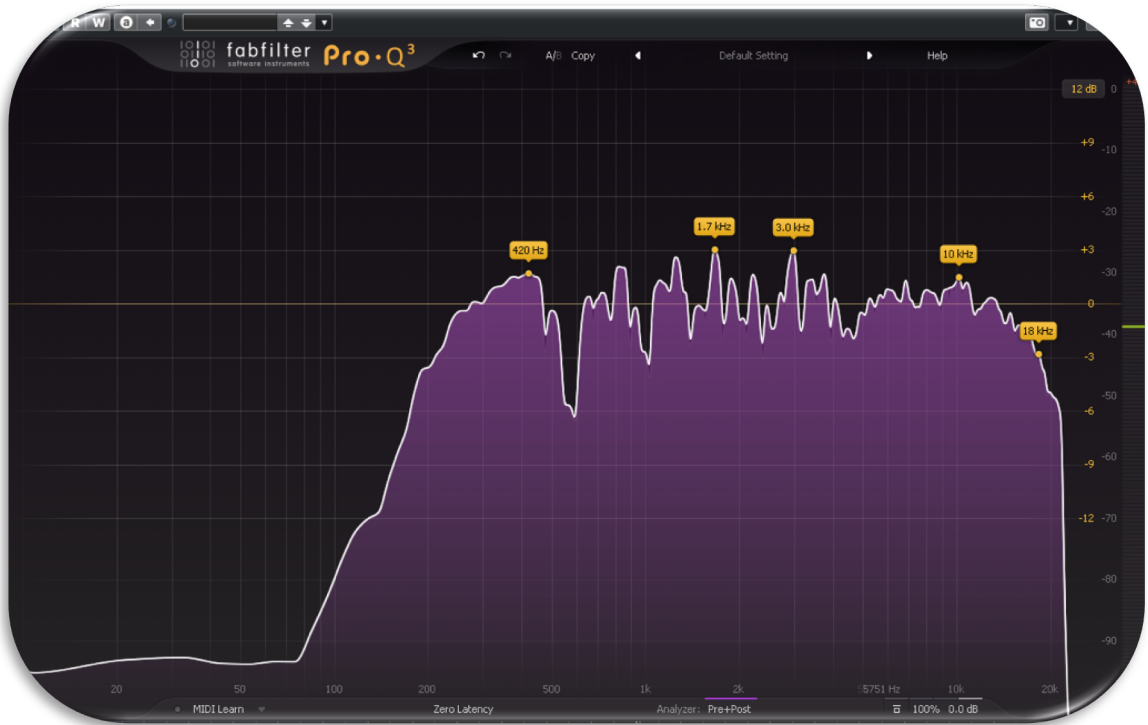
Picture 17. Spectrum analysis of the vocal with the Fabfilter Pro-Q3 plugin (Software)
