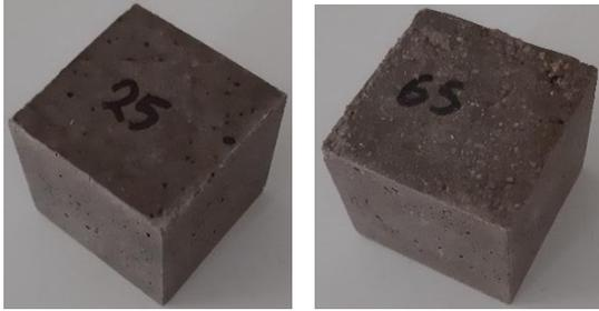
**Figure 4.** Incomplete consolidation of specimens preheated at 65°C.
