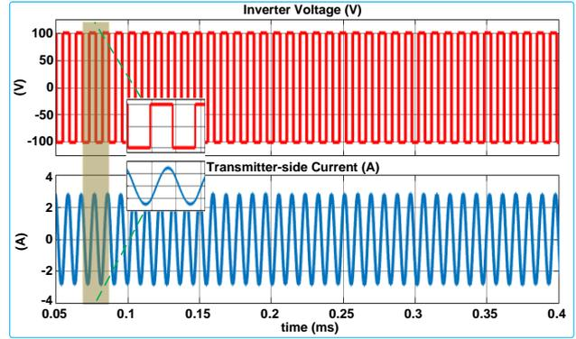
**Figure 7.** The waveforms of the inverter voltage and transmitter-side current.
