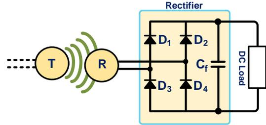
**Figure 5.** The single-phase uncontrolled rectifier circuit scheme.
