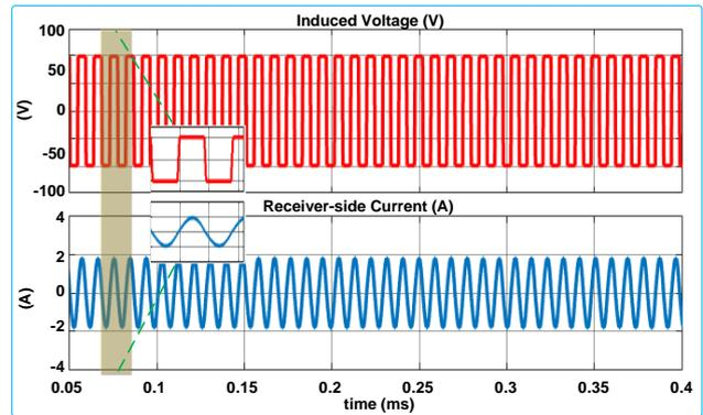
**Figure 8.** The waveforms of the induced voltage and receiver-side current.
